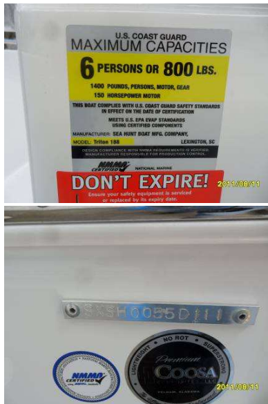
Sample builder's label and HIN on the left and ABP below
